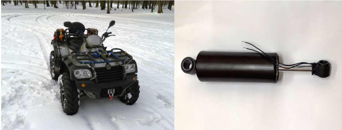
Fig. 1. Elements of semi-active vibration control system: a) experimental vehicle, b) magnetorheological damper
