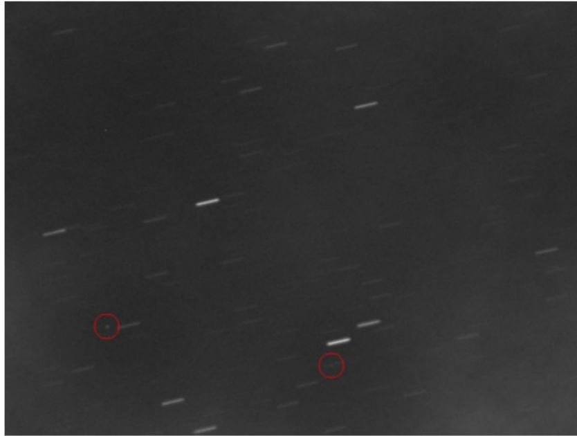
Fig. 1. An example image (out of a five-image sequence) showing the satellites that should be detected (annotated using red circles). All other objects should be filtered out as they would be the false positives
