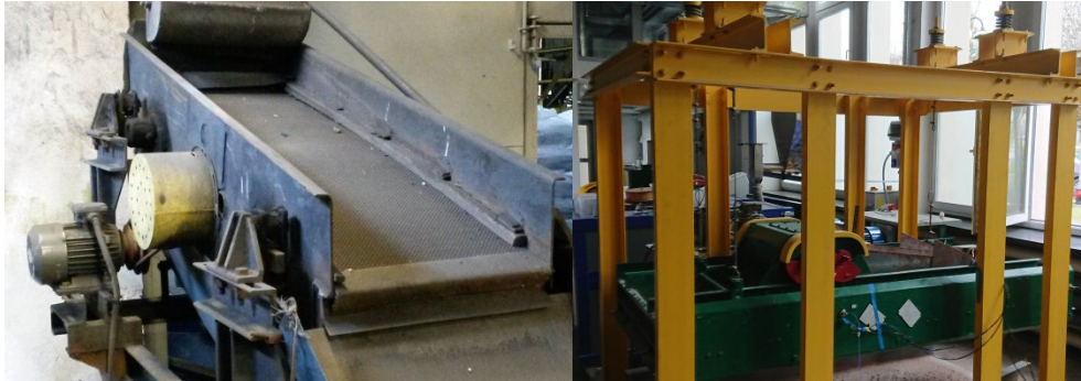
Fig. 1. Different constructions of screen suspension: a) riddle based on a spring suspension, b) riddle suspended on a spring suspension
