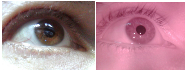
Fig. 1. The same eye image recorded by the same digital camera with and without IR filter (Genius FaceCam 2025 with IR filter switch). It is visible that iris and corneal reflections are much easier to find on the IR image
